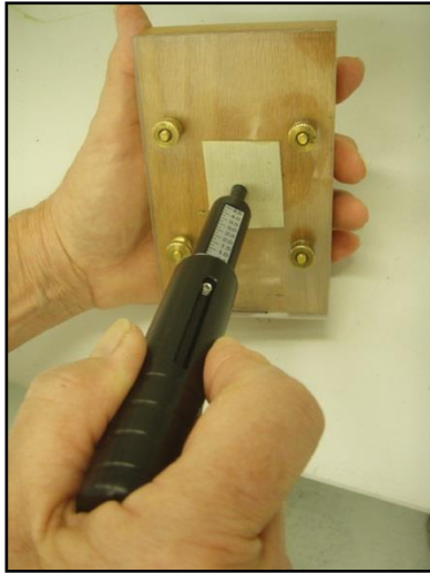
Fig. 4. Central American Tillandsia utriculata leaf sample being tested for toughness using a penetrometer.
